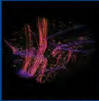
Chrysotile Asbestos CS Dispersion Staining Colors
